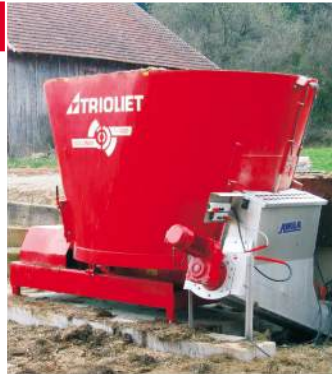
Single auger system for feeding into semi-sub soil digesters.
