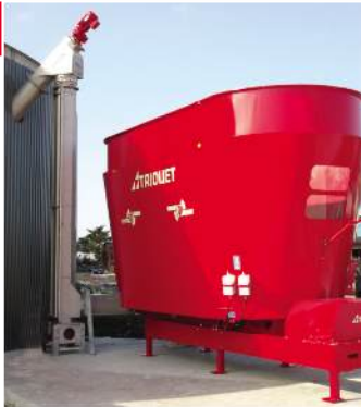
Triple auger system for feeding into standing digesters.
