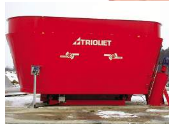
Standing auger system for feeding into sub soil digesters.
